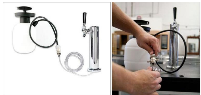
Connect the cleaning hose with its gasket
