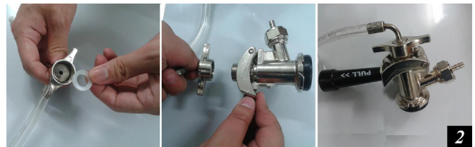
2 Connect the beer line to the coupler
